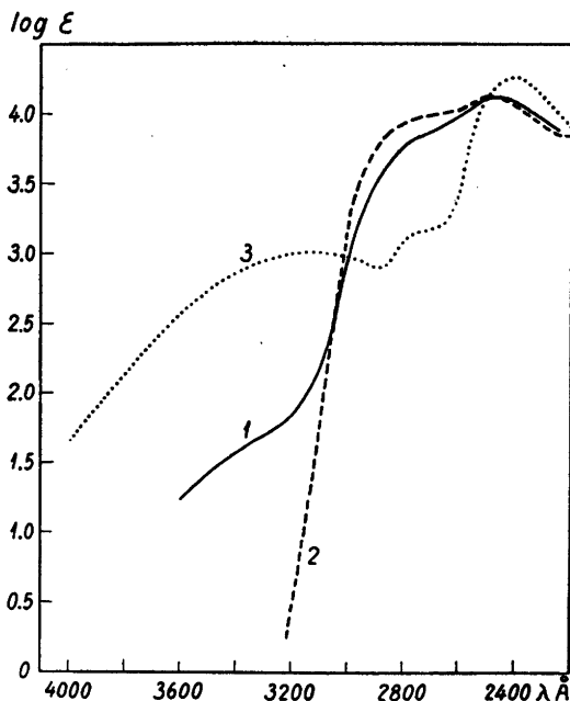
Fig. 2. 1) 1-Phenyl-3-methyl-5-pyrazolone ( 2.4 \cdot 10^{-3} , 2.4 \cdot 10^{-4} and 2.4 \cdot 10^{-5} M solutions) and 1-phenyl-3,4-dimethyl-4-bromo-5-pyrazolone ( 2.3 \cdot 10^{-3} , 2.3 \cdot 10^{-4} and 2.3 \cdot 10^{-5} M solutions) in 55 % ethanol measured 25 hours after the preparation of the solution. 2) 1-Phenyl-3,4-dimethyl-5-pyrazolone in ethanol ( 2.1 \cdot 10^{-2} , 4.5 \cdot 10^{-3} , 4.5 \cdot 10^{-4} and 4.5 \cdot 10^{-5} M solutions). 3) 1-Phenyl-3,4-dimethyl-4-bromo-5-pyrazolone in ethanol ( 4.0 \cdot 10^{-3} , 4.0 \cdot 10^{-4} and 4.0 \cdot 10^{-5} M solutions).
